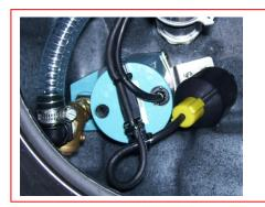
Connect the Female Garden Hose Fitting end of the Pump-out Hose to the outlet fitting on the back of the recovery tank. Place the other end of the pumpout hose in a sanitary drain.
