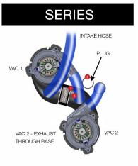
Connect Vac 1 exhaust hose to Vac 2 intake port
