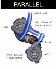
Connect Vac 1 exhaust hose to base exhaust port
