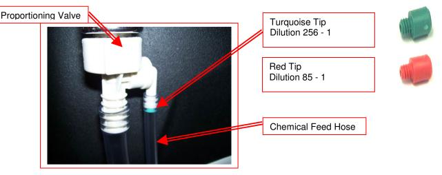
**Metering Tip Kit (Hydro-Force Item# PDE001)** contains 14 different colored metering tips, allowing dilution rates from 11:1 up to 427:1. Refer to the chart below to select the tip that meets the dilution rate for your chemical application.
