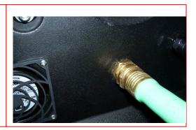
If not using the waste pump-out, the pump-out hose does not need to be connected. When the recovery tank fills during cleaning, the float assembly in the vacuum inlet filter will rise and will automatically shut off the vacuum air flow to prevent the recovery tank from overfilling and waste water from getting into the vacuums. When this occurs:
