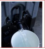
Drain water from Recovery Tank
