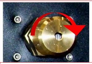
To increase the solution pressure, turn the regulator knob clockwise.
