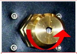
To decrease the solution pressure, turn the regulator knob counter-clockwise.
